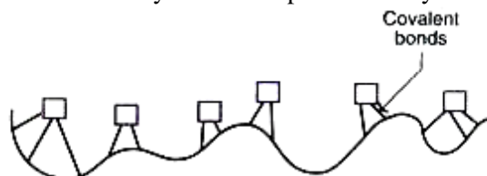
Fig. 21.5 : A general representation of immobilization of enzymes by covalent binding (Note : coloured blocks represent enzymes).
